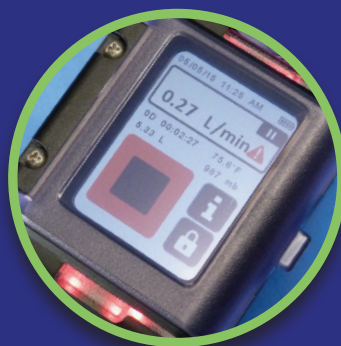
Flow fault and auto-restart
