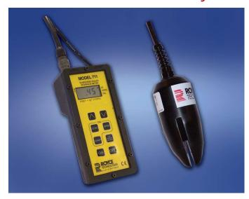
The Royce Model 711 Portable Suspended Solids/ Interface Level Analyzer is a rugged, waterproof instrument designed for the rigors of remote sampling. The meter provides reliable operation in waste treatment plants, rivers, lakes and other aqueous systems. The meter will read in either grams per liter when in the suspended solids mode or relative density percentage while in the interface level mode of operation.
